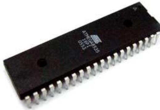
**Gambar Mikrokontroler ATmega8535**
